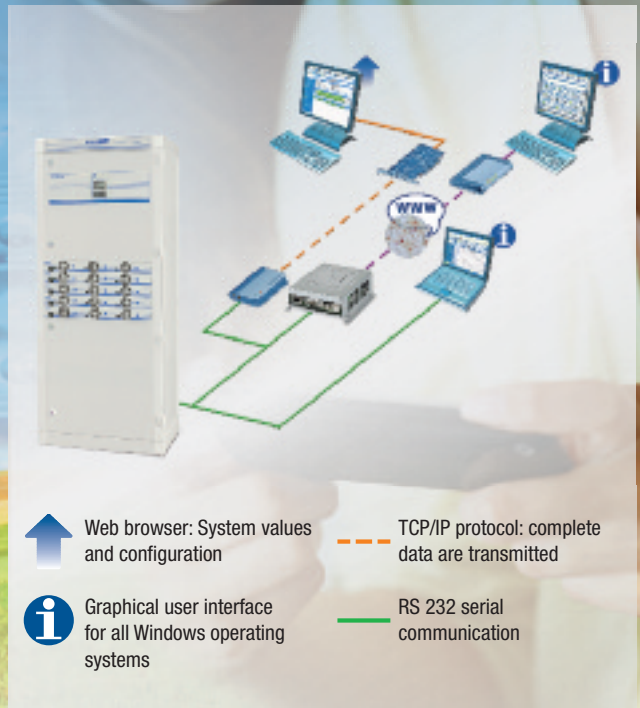
Fig. 9: MCU 2500 remote monitoring system
